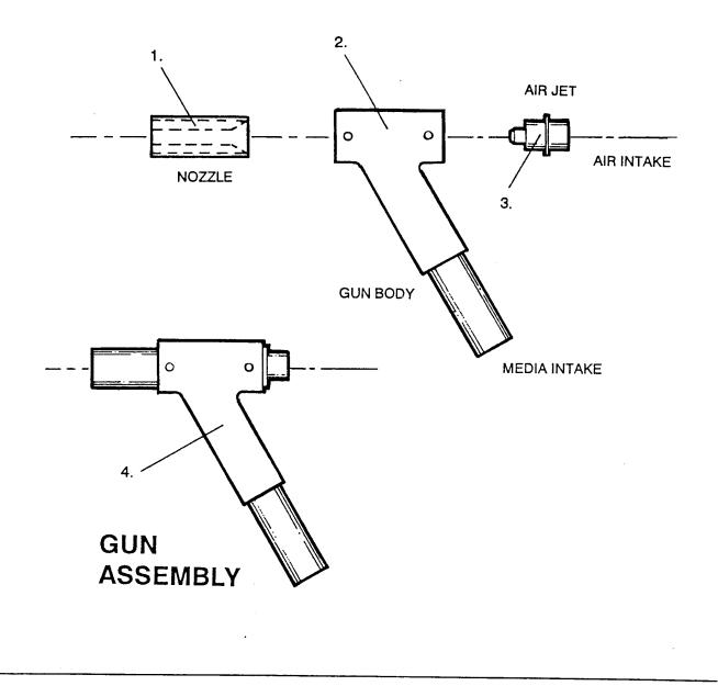
This blast gun is designed to create a static vacuum. This vacuum draws abrasive through siphon tube and abrasive hose into gun body, where compressed air pushes media through blast nozzle.
